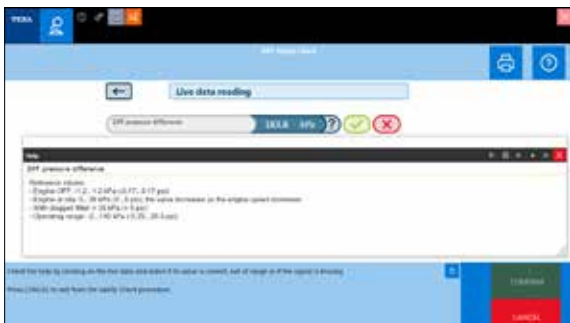
Error parameter reading with help sheet and component sheet
