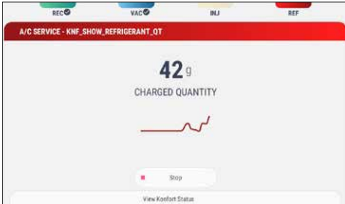
«Refrigerant charge» phase: the station charges the correct amount of gas into the vehicle system.
