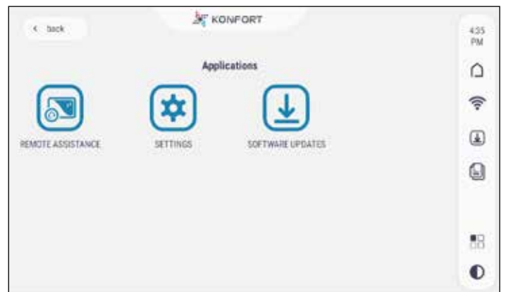
Applications page: to request remote assistance, access the settings, and check for updates.
